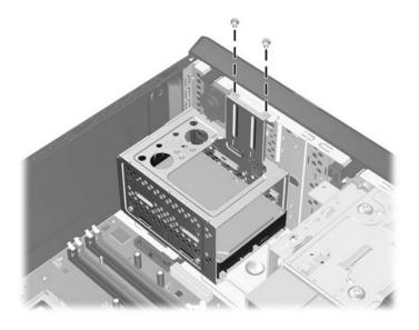
7. Push down the latch on the side of the hard disk drive cage (1), then slide the hard disk drive cage away from the bottom of the chassis (2) as shown below.
